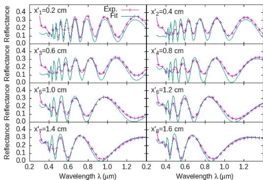
**Fig. 10.** Reflectance spectra at different positions ( $x'_n = 0.2 - 1.6$  cm,  $y = 0.74$  cm) on sample  $S_3$  ( $I_3 = 20$  mA) (Fig. 6). We show experimental results and results fitted through equations (18) and (19).
