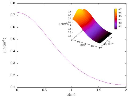
**Fig. 5.** Normalized current density  $j_\perp(x, y, 0)/I$  for a system as in Figs. 1 and 4 for a cell of length  $a = 2.01 \text{ cm}$  and width  $b = 1.48 \text{ cm}$ , with the surface of the electrolyte at a height  $c = 1.0 \text{ cm}$ , with a point-like electrode at  $r_0 = (0.2 \text{ cm}, 0.74 \text{ cm}, 0.9 \text{ cm})$ , calculated through Eq. (16) along the center line  $y = 0.74 \text{ cm}$ . Inset: current over the whole surface.
