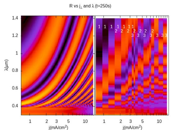
**Fig. 13.** Reflection  $R$  of a PS film as a function of the current density current  $j_{\perp}$  and wavelength  $\lambda$  for an etching time  $t = 250$  s. Theory (left panel) and experiment (right panel, see text). We indicate with the numbers 1, 2, 3 the data corresponding to the corresponding samples  $S_1$ ,  $S_2$  (shifted, see text) and  $S_3$ .
