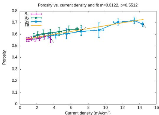
**Fig. 11.** Porosity vs. current density for the three samples  $S_1$ ,  $S_2$ ,  $S_3$ . The arrows point to data that correspond to position  $x'_1 = 0.2$  cm (see text). We include a linear fit of the form  $p = mj_{\perp} + b$  with parameters  $m = (0.0122 \pm 0.001) \frac{\text{cm}^2}{\text{mA}}$  and  $b = 0.551 \pm .005$ .
