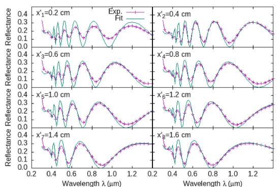
**Fig. 9.** Reflectance spectra at different positions ( $x'_n = 0.2 - 1.6$  cm,  $y = 0.74$  cm) on sample  $S_2$  ( $I_1 = 10$  mA). We show experimental results and results fitted through equations (18) and (19).
