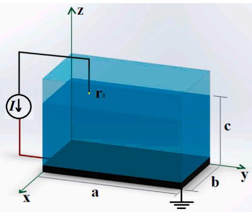
**Fig. 1.** Prism shaped electrolytic cell with a rectangular base of sides  $a$ ,  $b$  filled with electrolyte up to a height  $c$ . The walls of the cell are insulating and the bottom is completely covered by the sample, which is assumed to be a good conductor. The tip of the electrode is a thin insulated wire with just the tip uncovered and located at  $r_0 = (x_0, y_0, z_0)$  within the liquid. The current flows through the electrolyte from the sample to the tip.
