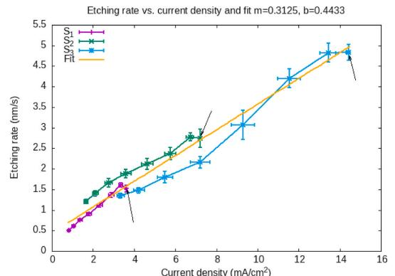
**Fig. 12.** Etching rate vs. current density for three samples  $S_1$ ,  $S_2$ ,  $S_3$ . The arrows point to data that correspond to position  $x'_1 = 0.2$  cm (see text). We include a linear fit of the form  $v = mj_{\perp} + b$  to the data with parameters  $m = (0.312 \pm 0.017) (\text{cm}^2/\text{mA})(\text{nm}/\text{s})$  and  $b = (0.44 \pm 0.09) \text{ nm}/\text{s}$ .
