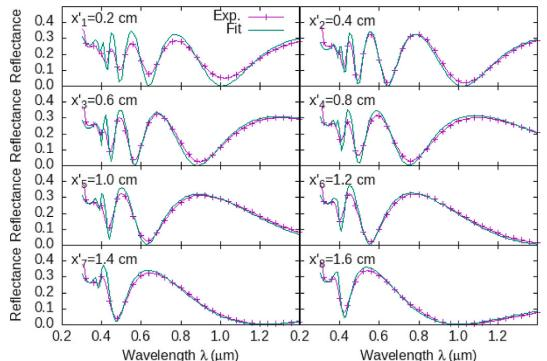
**Fig. 8.** Reflectance spectra at different positions ( $x'_n = 0.2 - 1.6$  cm,  $y = 0.74$  cm) on sample  $S_1$  ( $I_1 = 5$  mA). We show experimental results and results fitted through equations (18) and (19).
